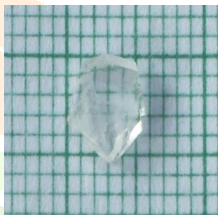
Fig. (c) As grown crystal of 2 mole % KI doped ZTS
