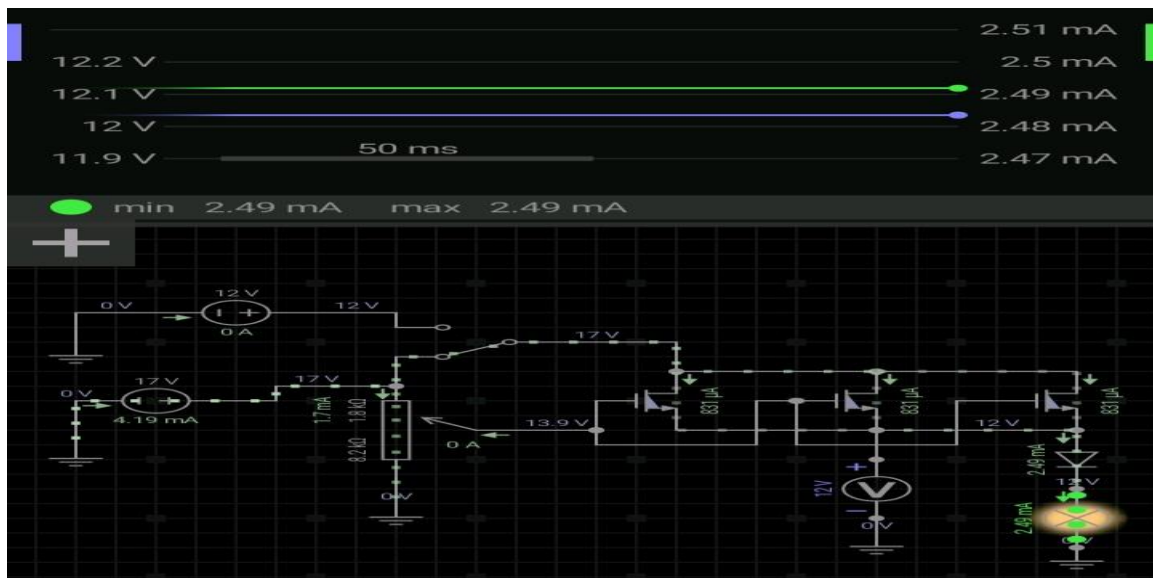
Fig 3 - When Solar Panel Is Powering the Circuit
