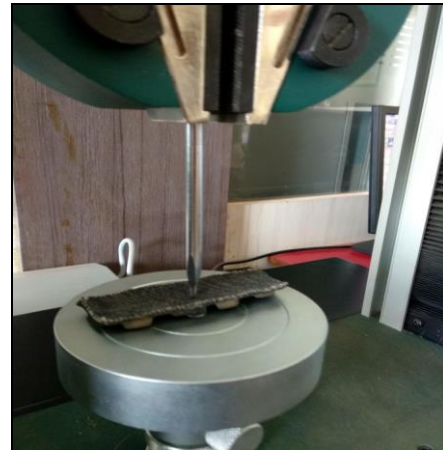
Fig. 3. Slow rate penetration test setup
