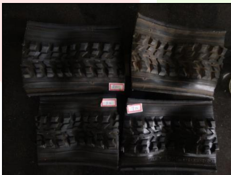
Fig. 2. Specimens with respective compositions a.5wt%, b. 3wt%, c.7wt%, d.WC
