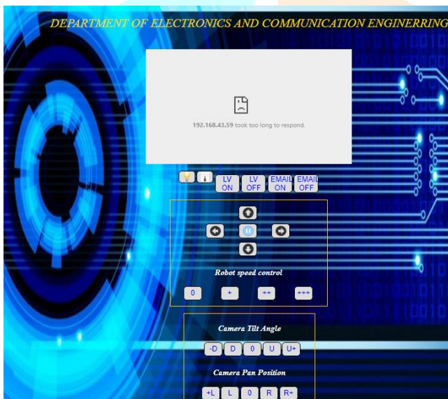
Figure 12: HTML Web Page for Remote Control
