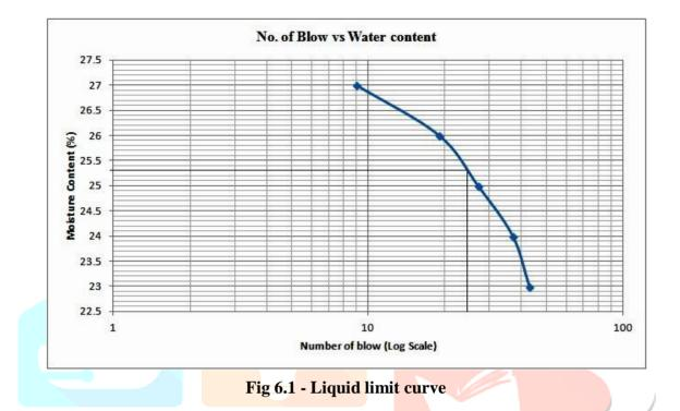
Liquid Limit is the water content at 25 blows. It can be seen from the curve that
