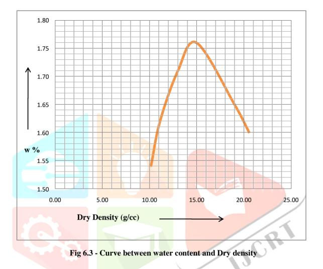
**Result:** The water content of the sample = **15% (approx)** and Draw a curve between water content and dry density
