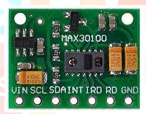
The sensor is integrated pulse oximetry and heart-rate monitor sensor solution. It combines two LED's, a photodetector, optimized optics, and low-noise analog signal processing to detect pulse and heart-rate signals. It operates from 1.8V and 3.3V power supplies and can be powered down through software with negligible standby current, permitting the power supply to remain connected at all times.
