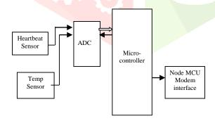
[Fig 1] Block Diagram of the system The square chart comprises of five fundamental parts. These are:
