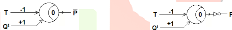
Fig. 13(a) Threshold logic gate of P Fig. 13(b) Complement of Fig. 14(a)
