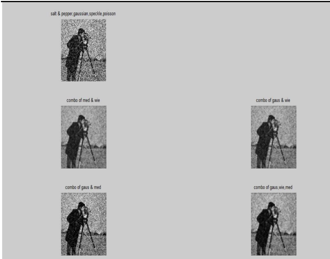
Fig 4.5.1: The input image (cameraman.tif) is noised with combination of all the 4 noises i.e (salt & pepper + Gaussian + Speckle + Poisson) noise. Here the noisy image acts as an input image to the filters. Noise is added externally to note the changes. The noised image is denoised using combination of 2 and 3 filters i.e (Gaussian + wiener), (Gaussian + Median), (Median + Wiener), (Gaussian + Median + Wiener).
