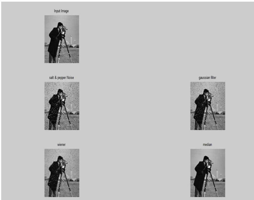
Fig 4.1.1: The input image (cameraman.tif) is noised with salt and pepper noise. Here the noisy image acts as an input image to the filters. Noise is added externally to note the changes. The noised image is denoised using Gaussian, wiener, median filter.
