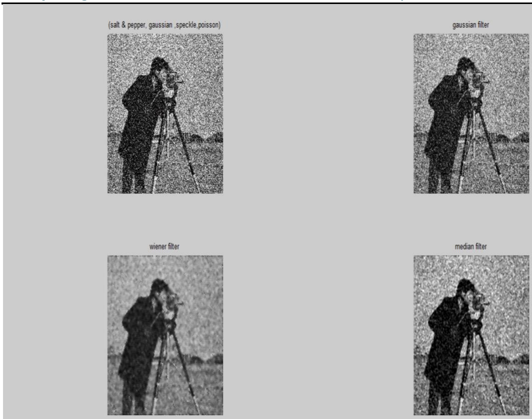
Fig 4.2.1: The input image (cameraman.tif) is noised with combination of all the 4 noises i.e (salt & pepper + Gaussian + Speckle + Poisson) noise. Here the noisy image acts as an input image to the filters. Noise is added externally to note the changes. The noised image is denoised using Gaussian, wiener, median filter.
