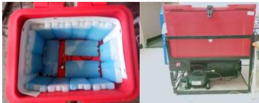
Fig.No.1 (a) PCM enclosed in cooling pack (b) Actual set-up front view
