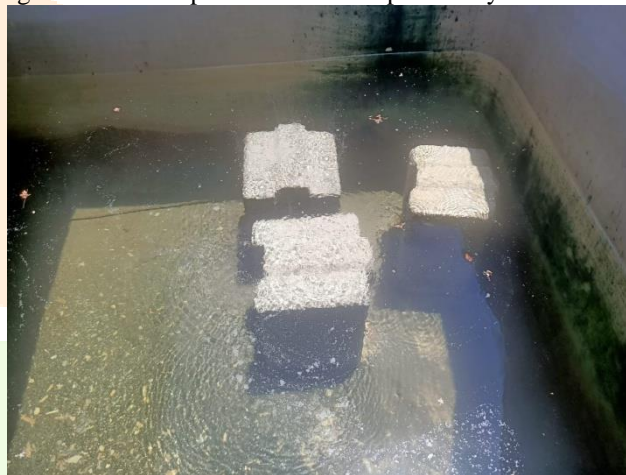
FIG. 3 WATER ABSORPTION TEST
