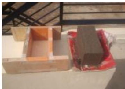
Fig.4 Papercrete mould and brick
