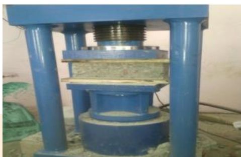
Fig. 5 Compression test on papercrete bricks
