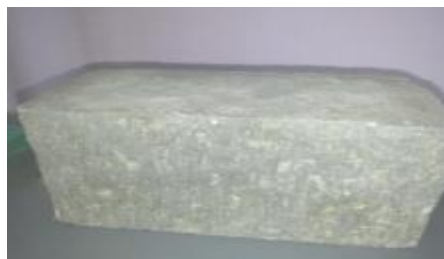
Fig.6 Specimen after Efflorescence Test
