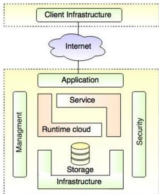
Fig- Graphical View of Cloud Computing Architecture.
