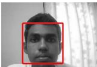
Figure 5: Face detected from the frame using Haar Cascade Classifier The geometrical properties of human face are computed, in the face image as in Figure 6 shows that it is extracted from the video frame and the left and right eyes are separated.
