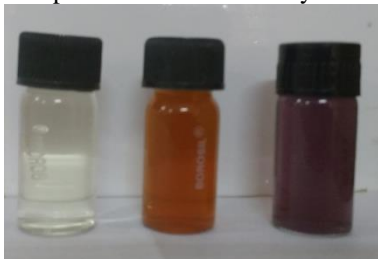
Fig.2 Images of plant extract (light colour), AgNPs (brown colour) and AuNPs (Pink colour)
