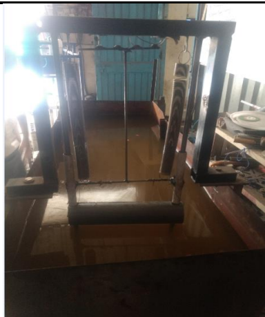
Fig.-3. Actual working model of VIV system
