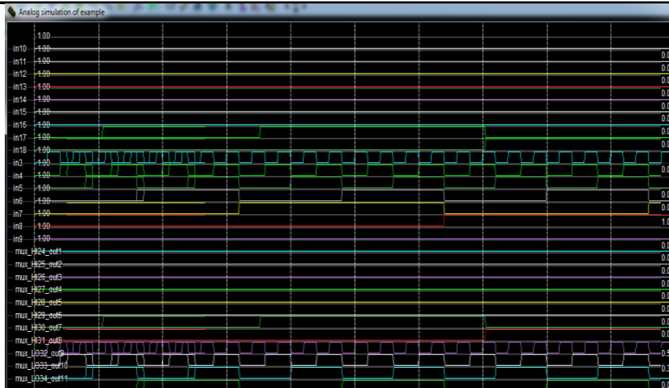
Fig.8. Simulation results of the proposed Data Comparator in 90nm Technology.
