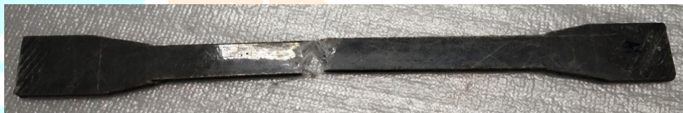
Fig.3 Specimens before Tensile Test
