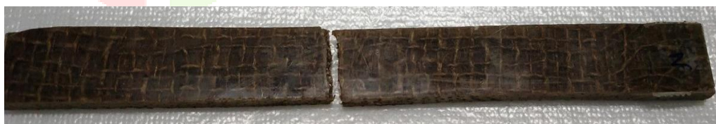
Fig.6 specimen after flexural test
