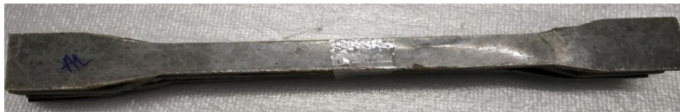
Fig.3 Specimens before Tensile Test
