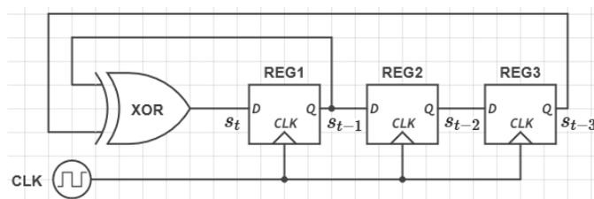
Figure.3 LFSR Circuit
