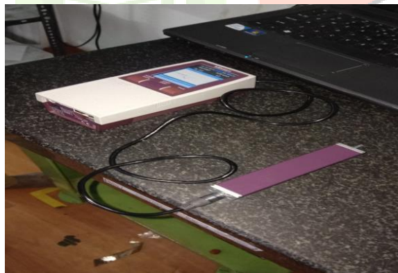
Fig.4 Talyor Hobson Talysurf device
