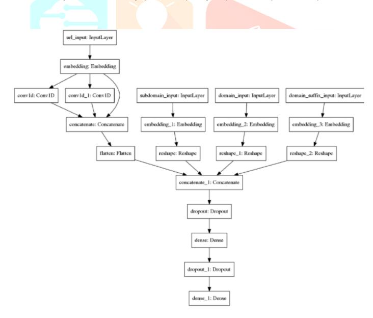
allowing the complete model to output binary classifications (i.e a Malicious or legitimate URL). Figure above shows the architecture of the CNN-1D model used in this work.
