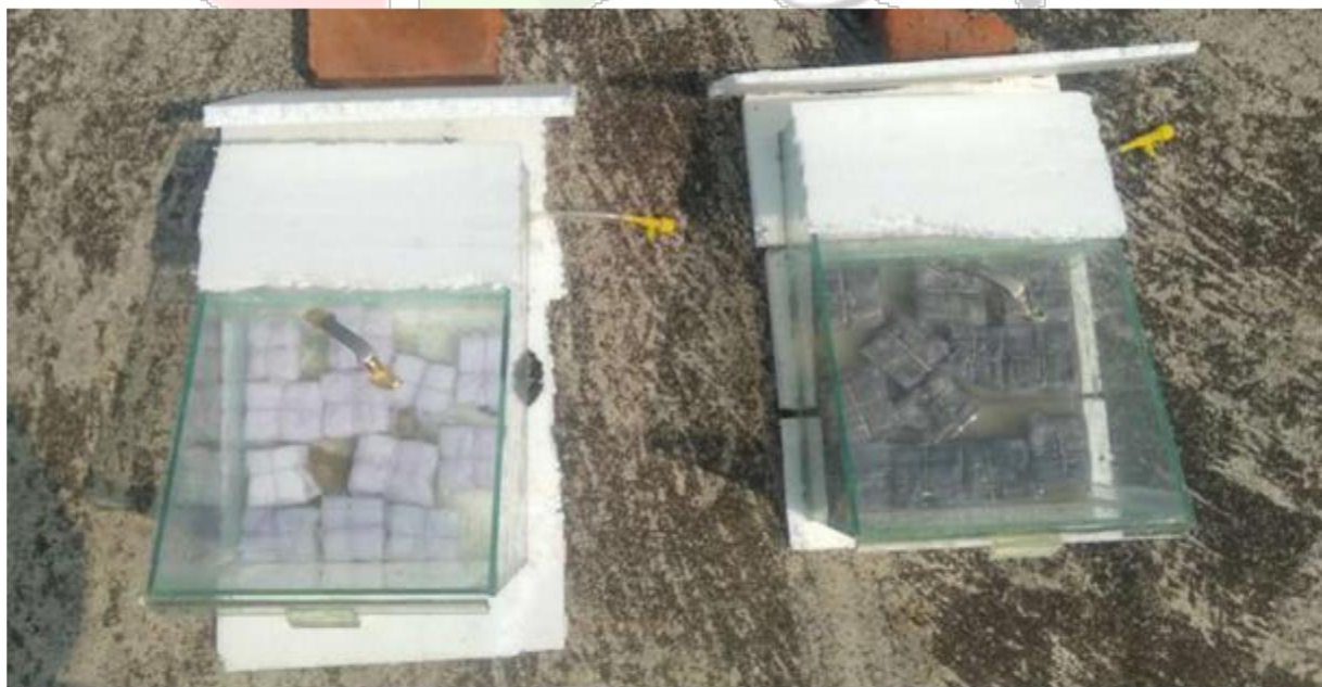
Fig.3. Solar still using GO coated and uncoated cotton
