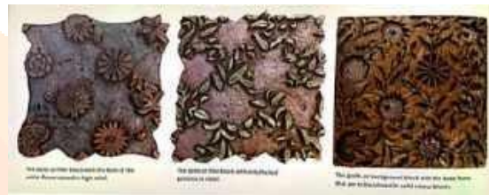
Figure 11: Different Blocks with same design, 1. Filler block with entire flower raised, 2. Filler block with only lead pattern is raised, 3. Background block
