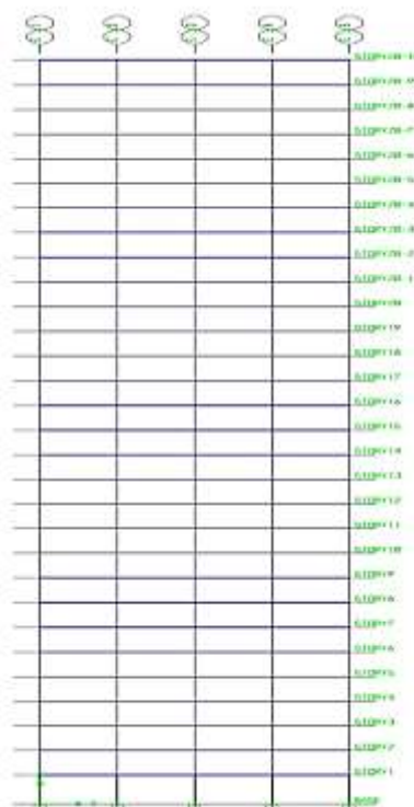
Figure 3.9.3.4 Elevation of 30 - Storey building without strut
