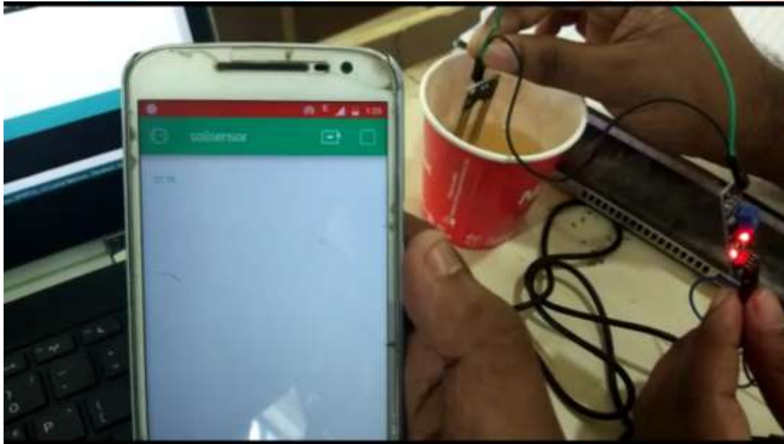
Fig 9: Soil moisture content displayed on blynk app using adafruit library programming with Arduino
