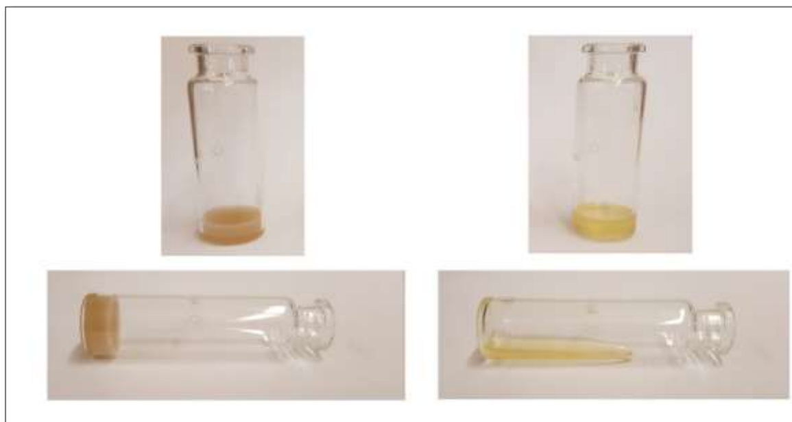
Figure 6.4: Effect of PPDs with blended alkyl esters to model oils
