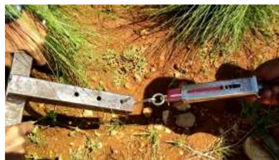
Fig 3.1(b): Spring Balance reading = 25Kgs (For Wet Land)
