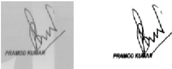
Fig 6: Process of binarization of a sample of a signature
