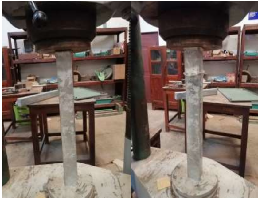
Fig -10: ISCFDST Specimen Before Loading Fig -11: ISCFDST Specimen After Loading
