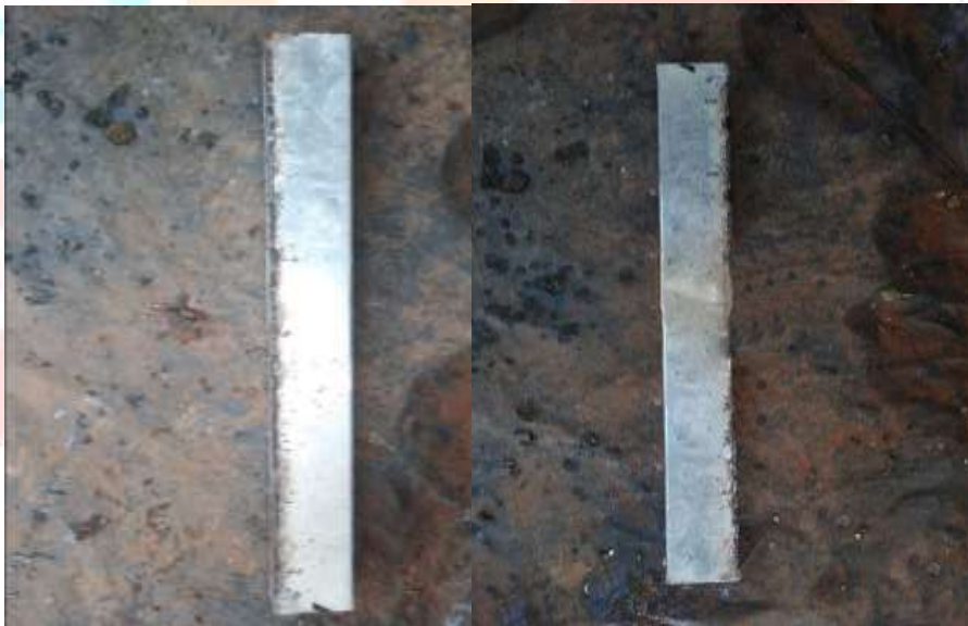
Fig -11: ICHCFDST Specimen Before Loading Fig -12: ICHCFDST Specimen After Loading
