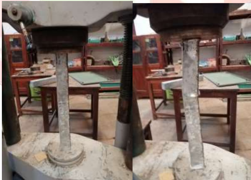
Fig -8: ICCFDST Specimen Before Loading Fig -9: ICCFDST Specimen After Loading
