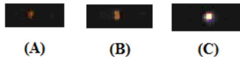
Figure 6: Photographs showing the light emission recorded by camera at 10 V for the devices made on set C viz. (A) ITO/MEH-PPV/Al, (B) ITO/MEH-PPV/LiF:Al and (C) ITO/MEH-PPV/Alq 3 /Al.
