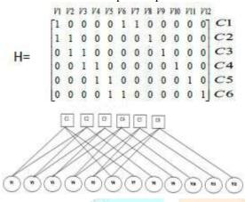
The nodes c1, c2, c3... are known as check nodes, these represent the columns and the nodes v1, v2, v3... are known as variable nodes, these represent the rows of the parity check matrix (H- matrix) [5].
