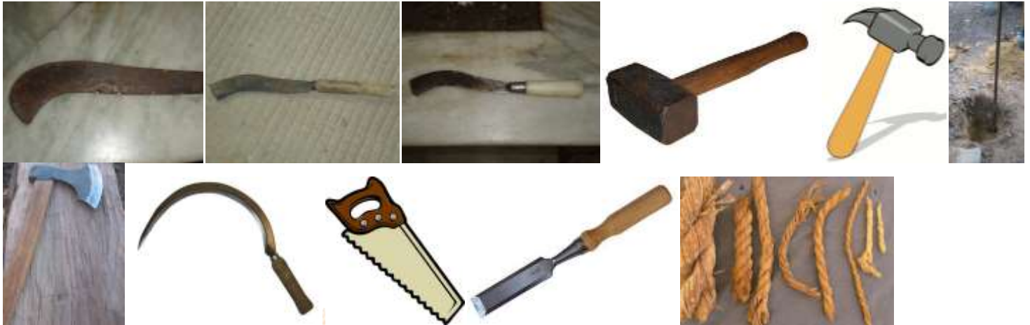
Fig : 35 Construction tools - daa, kotari, haturi(Normal hammer), claw hammer, khonta, kuthar (Axe), kasi(Sickle), korat(Shaw), Botali(Chisel), rosi(Jute Rope)
