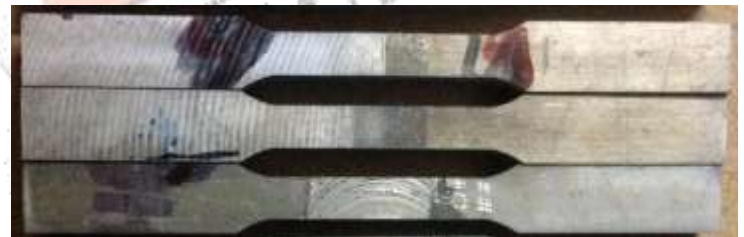
Fig.4 Specimen Prepared on EDM wire cut
