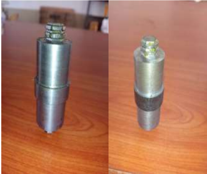
Fig.2 Showing Tools used 1) Tool with Hexagonal Pin with Hexagonal ring 2) Tool with Circular Pin with Circular rings.
