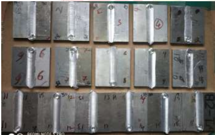
Fig.3 Friction Stir welded Specimen
