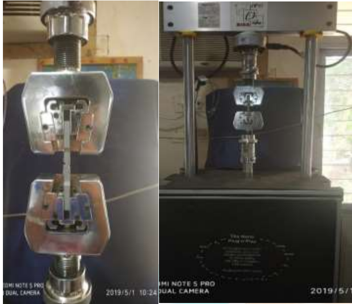
Fig.5 Mounted Tensile test specimen on Digital Hydraulic UTM.
