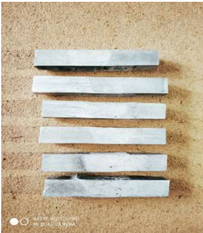
Fig.7 Specimen Prepared to perform Microhardness Test
