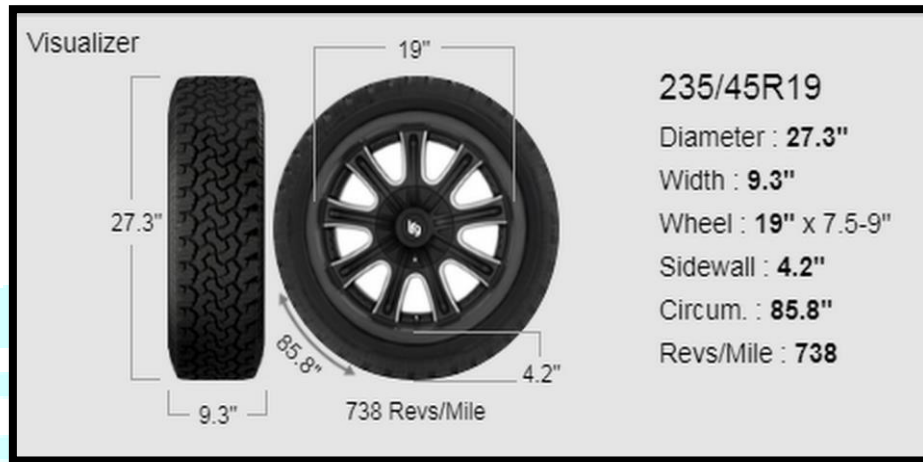
Fig 11: Standard tyre size [5][13]
