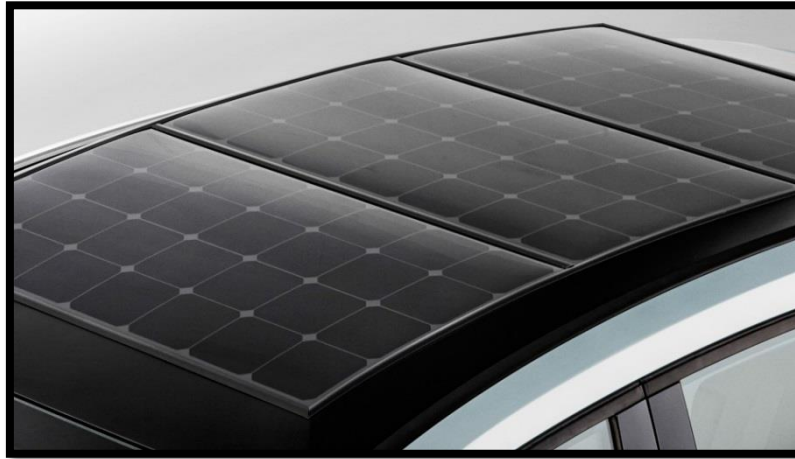
Fig 2: Solar Panels (group of solar cells) on the roof of a solar powered vehicle [11]
