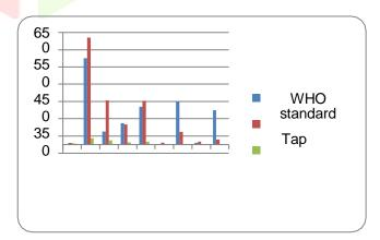
The WHO has suggested a limiting value of 500 ppm of TDS for potable water. While the minimum TDS for the tap water samples under present investigation is 621 ppm whereas the highest value of TDS has risen to 1390 ppm. Such high values of TDS must be reduced by suitable method to reinstate the potability of water.
