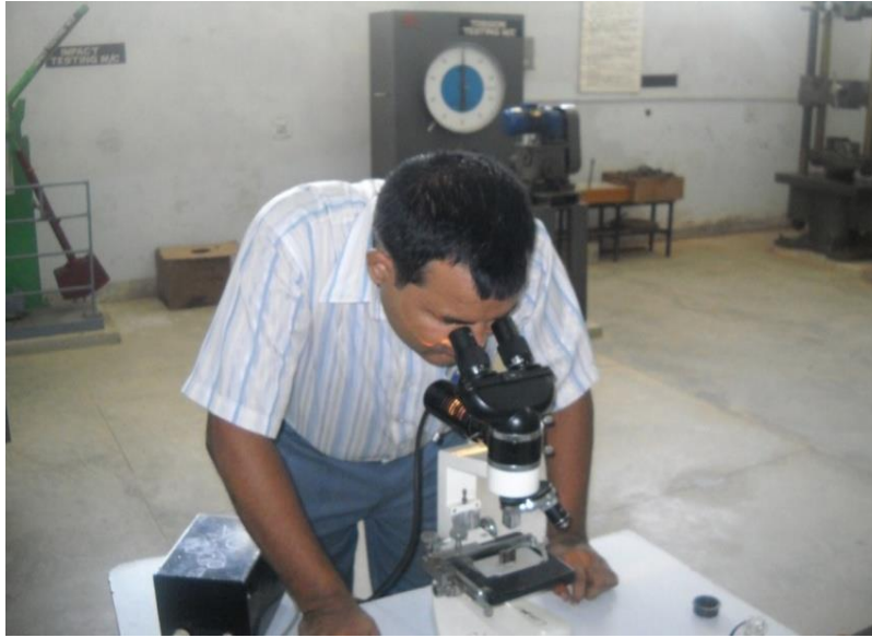
Figure 1: Measurement of weld bead dimensions using metrological microscope
