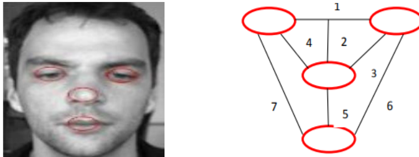
Figure 7- Face Feature Calculation
