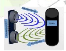
The ultrasonic receiver would detect the reflected wave and stop timer. After calculating the distance, the information will send to the Arduino and then, the headset produces the voice. In this system, the distance is measured between the object and the Dark Light kit, the information is sent from the sensor to the Arduino board. The operation of the Dark Light system is composed of an ultrasonic sensor, an Arduino Nano. The ultrasonic sensor senses the
