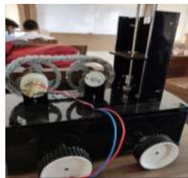
Fig7.3: Goods loading vehicle with lead screw mechanism
