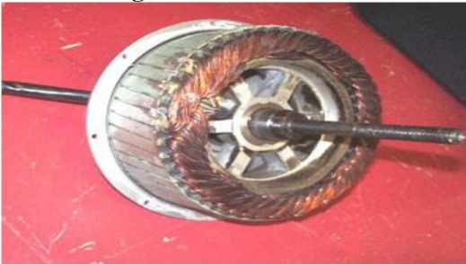
Fig 2: Hub Motor Rotor
