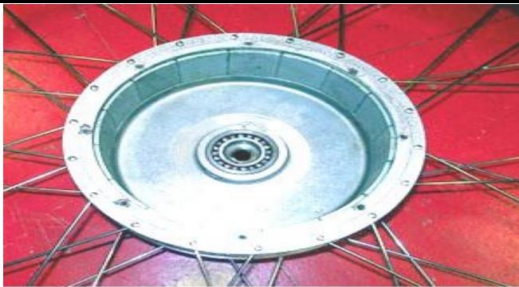
Fig 2: Hub Motor Rotor
