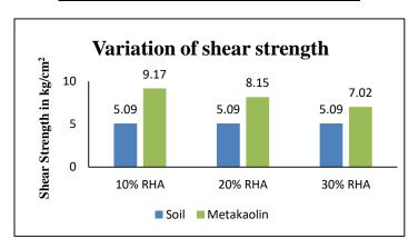
**Fig 4.1:** The above graph indicates the variation of shear strength of cohesive soil and soil replaced by 10%, 20% and 30% of rice husk ash with addition of 20% metakaolin
