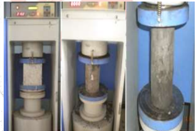
Figure 1: Compression Test on Cube and Cylinders
