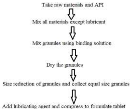
Fig: 2. Method of preparation of granules (one step process)
