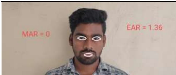
Fig.8. EAR and MAR value detected on open eye.
