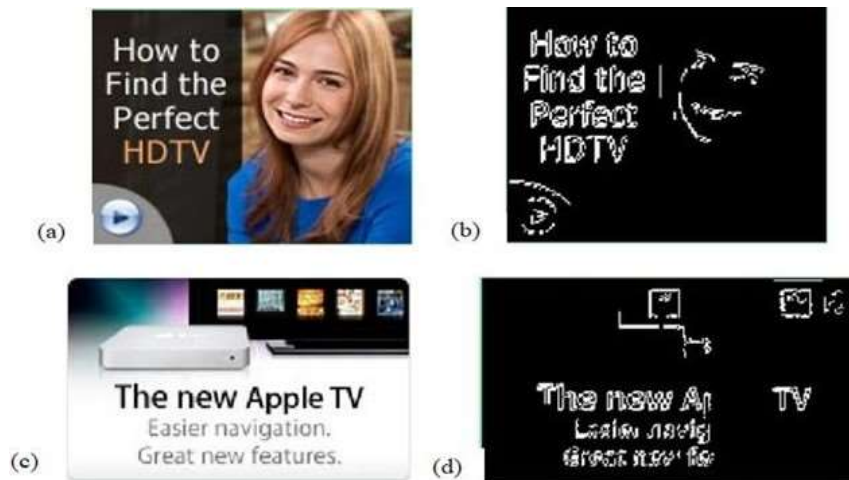
Fig.3: Extraction process of Connected Component Algorithm- (a) And (c) are original images, (b) and (d) respective output
