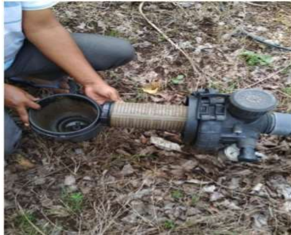
Figure 1: Existing Filter System Clean by Manual Method
