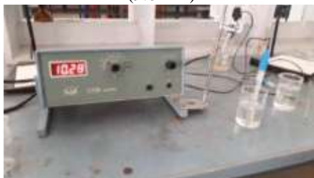
Fig.13 Test Case: ASH Water Testing (10.28PH)
