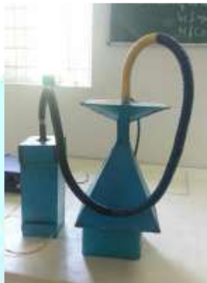
Fig.5 Incinerator and Venturi Scrubber
