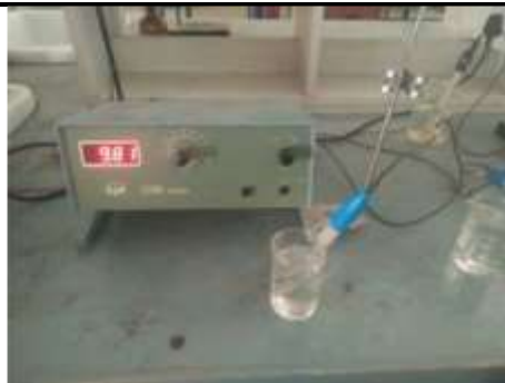
Fig.11 Test Case: Salt Water PH Testing (9.81PH)
