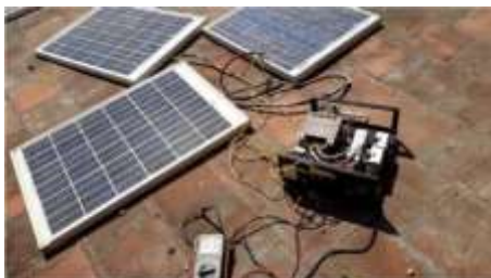
Fig.7 Test Case: Testing Solar Panel Parallel Connection
