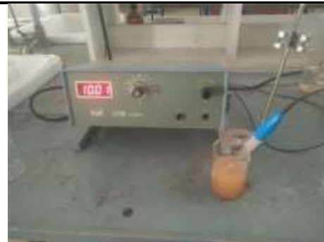
Fig.12 Test Case: Soil Water PH Testing (10.01PH)
