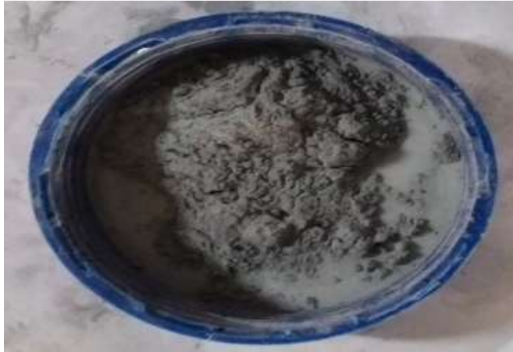
Fig.5 Mixed ratio of 95%Al and 5% B 4 C
