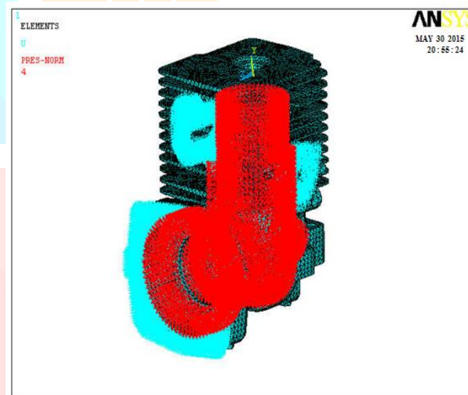
Figure 3.2 Boundary conditions applied for the engine block
