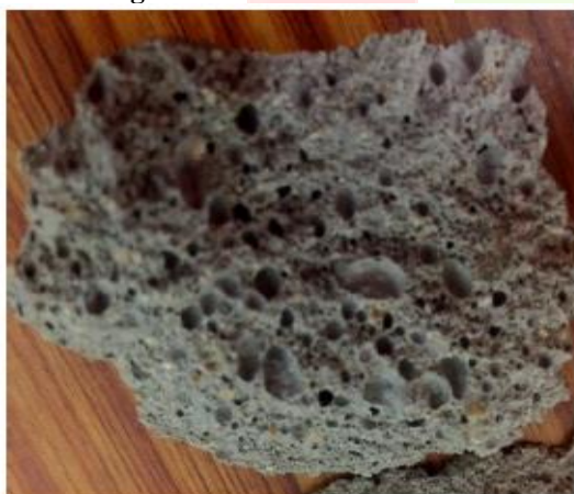
Figure 8 Internal Structure of Foam concrete block
