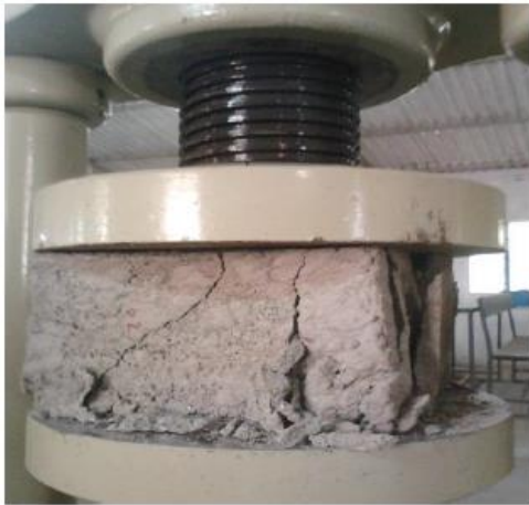
Figure 6 Crushed Foam Concrete Cube
